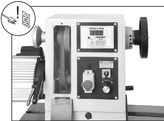
Figure 56. Belt access cover opened.
